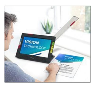
The **RUBY 10** video magnifier has a 10-inch touchscreen and three dedicated cameras. The **RUBY 10** can magnify letters, magazines, labels, and photos. The swing-out arm allows you to view items in your hand and write. When extended, on the speech model, the arm also enables full-page OCR. With a touch of a button, you can scan pages and have them read aloud to you. The third camera is dedicated to seeing objects at a short distance such as signs and menus on a wall.
